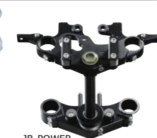
JB-POWER Milled Aluminum Fork Bridge [Triple Trees] φ38 Adjustable Offset 40/45mm ¥ 180,000.- Fixed Offset 45mm ¥ 150,000.- Black Finish + ¥ 5,000.-
